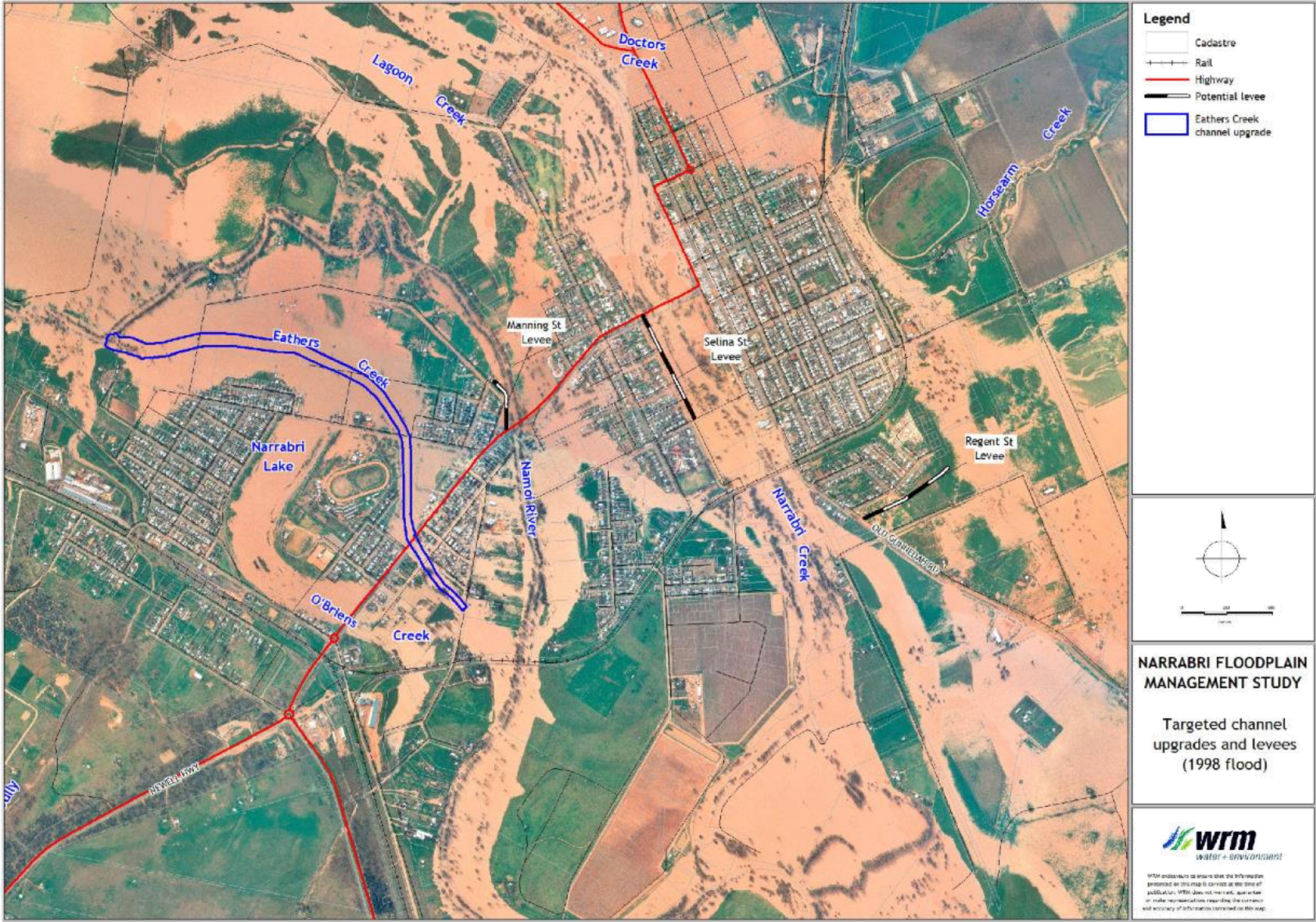
Figure 6.5 - Targeted channel and levees upgrade layout
