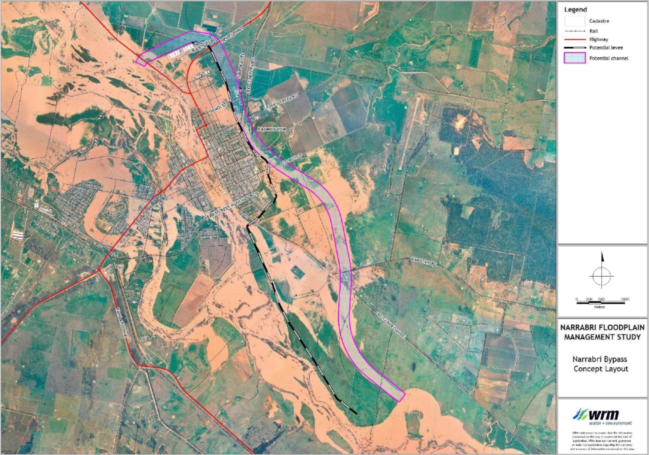
Figure 6.2 - Narrabri bypass concept layout (overlayed on 1998 flood extent)
